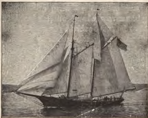
FIG. 389. A New England fishing-smack (a schooner) driven by sail power only. Vessels like this can and do go anywhere in the world.
